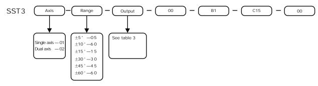
For example, if order a dual axis thermal shock-proof inclinometer, with range  $\pm 15^{\circ}$ , room temperature accuracy  $\pm 0.02^{\circ}$ , output RS422, 2 meters cable with plug, the model should be chosen as: SST302-15-G2-00-B1-C15-00
