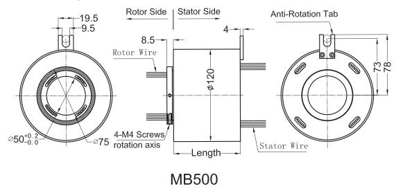
12 wires for one group color. from 13  $\dots$  24, repeat the same color as 1  $\dots$  12, indicated with number code pipe.
