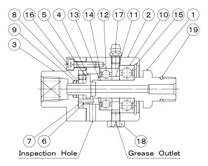
1) Rotor 2) Casing 3) Head 4) Seal Ring 5) Spring 6) Spring Pin 7) Fixing Flange 8 Buck-up Ring 90-ring 10 Ball Bearing 11 Spacer (12) Ball Bearing (13) Retaining Ring (14) Wave Washer (15) Retaining Ring (B) Cap Screw (1) Grease Nipple (B) Plug (Slotted Head Hex. Bolt) (9) O-ring
