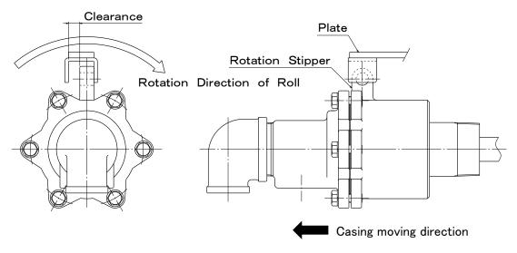
Note ) The seal face of the seal ring becomes worn over the course of operation time, and the casing moves in the arrow direction.
