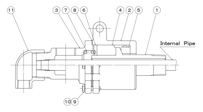
①Rotor ②Casing ③Head ④Carbon Bearing ⑤Seal Ring ⑥Washer ⑦Spring ⑧Gasket ⑨Hex. Bolt ⑩Spring Washer ⑪Elbow
