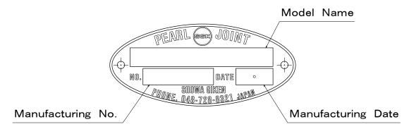
The nameplate attached to the product indicates the model name, manufacturing number, and manufacturing date.
