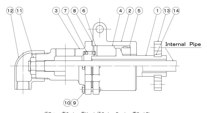
①Rotor ②Casing ③Head ④Carbon Bearing ⑤Seal Ring ⑥Washer ⑦Spring ⑧Gasket ⑨Hex. Bolt ⑩Spring Washer
