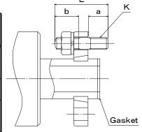
2. A duplex, stationary IP, flange connection product (NCF) is supplied with a lock nut (right-hand thread) used for securing the internal pipe to the product. The material of the lock nut is SS400.
