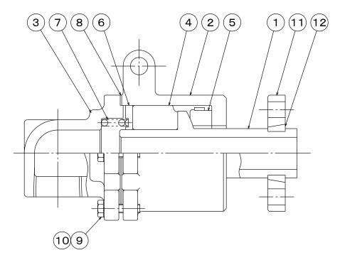
①Rotor ②Casing ③Head ④Carbon Bearing ⑤Seal Ring ⑥Washer ⑦Spring ⑧Gasket ⑨Hex. Bolt ⑩Spring Washer ⑪Rotor Flange ⑫Split Ring
