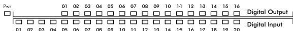
Fig. 6: LEDs on the front side of the device for monitoring (here: ZX20T)
