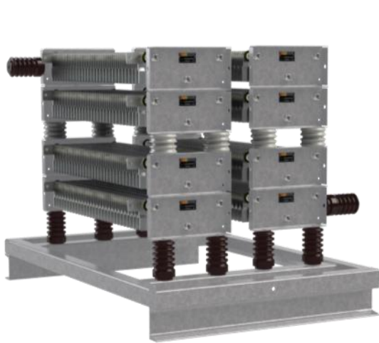
IPOO resistor: 14 Ohm. 500 Amp. -10 sec Insulation level: 12 kV.
