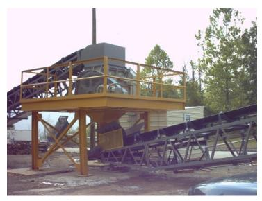
Used to detect small pieces of metal, the Bulk Pro Systems Model 5500 Tramp Metal Detector is well suited for rugged environments. It will detect both magnetic and non-magnetic metal and is not affected by most process materials. Proven dependable under adverse conditions such as dust, moisture and vibrations, Bulk Pro Systems Model 5500 provides years of trouble free reliable operations.
