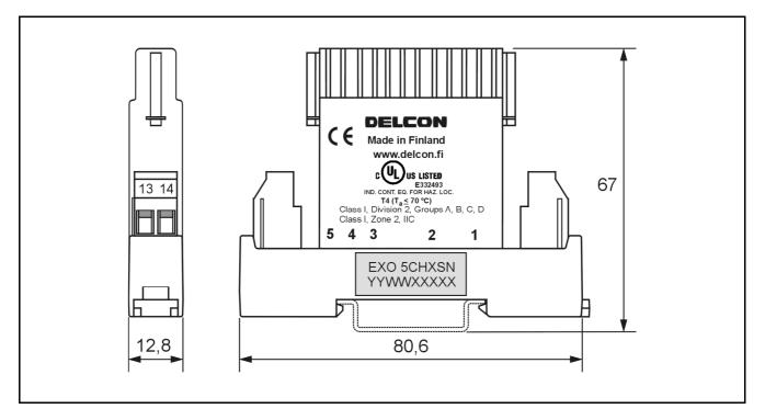
EXO 5CHXSN (dimensions in mm, nominal). Markings can be located differently by production lot. Parts of the markings are backside of the relay. Production lot number is marked to the socket (YY = year, WW = week, XXXXX = lot number).
