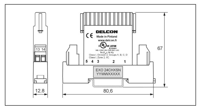
EXO 24CHXSN (dimensions in mm, nominal). Markings can be located differently by production lot. Parts of the markings are backside of the relay. Production lot number is marked to the socket (YY = year, WW = week, XXXXX = lot number).
