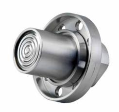
Diaphragm seals are designed to isolate the sensing element of pressure gauges and pressure switches from process fluids which may be corrosive, viscous, sedimentous and/or with a high temperature. The diaphragm is welded to the upper body, to ensure separation of filling fluid from process medium. The "in-line" diaphragm position enables deep cleaning of their surfaces. Flange clamping with metallic sealing guarantees the system against leakage at high process fluid temperatures and pressures.
