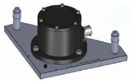
Adjustable base with micrometer screw is for carrying and fixing SST300 inclinometer of Accessories. When install SST300 device, user do not consider whether surface status, and can achieve to precise zero adjustment and quick installation by three-point adjustment via the micrometer screw.
